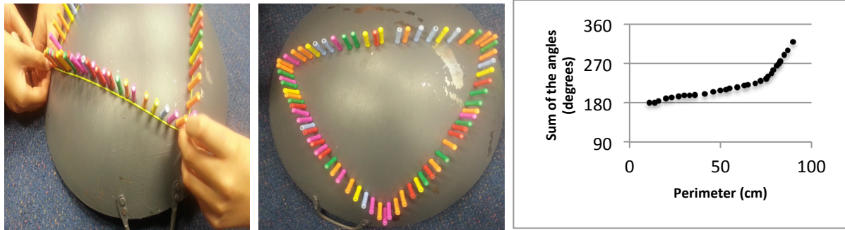
Figure 7(a). Students comparing the two methods of defining a straight line in curved space. Magnets are used to create sightlines. The stretched string confirms that this is the shortest path.
