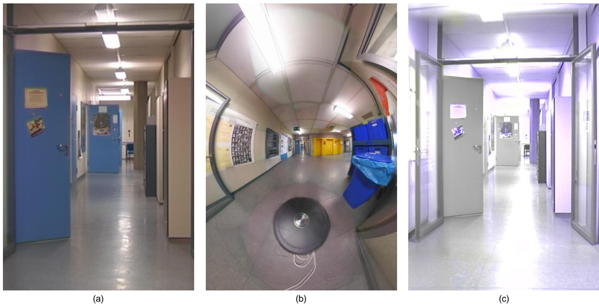
Figure 5.16: Image (a) shows the non-relativistic view, image (b) the apparent geometry for \beta = 0.99 , and image (c) completely relativistic rendering with \beta = 0.3 . The overall intensity in (c) is reduced to one half of that in (a) and (b) to avoid extreme clamping of the final RGB values.
